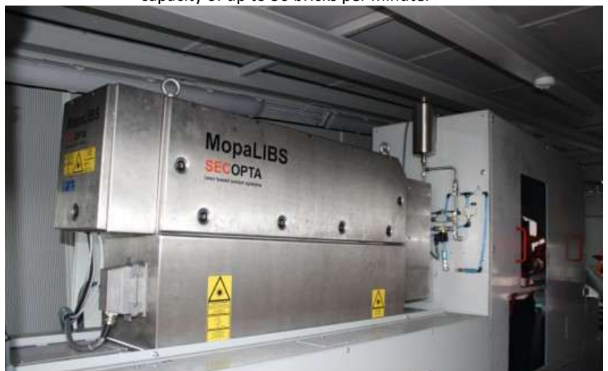
The MopaLIBS sensor is arranged above the conveyor belt that transports the material to be recycled. (Photo: Secopta analytics GmbH)
